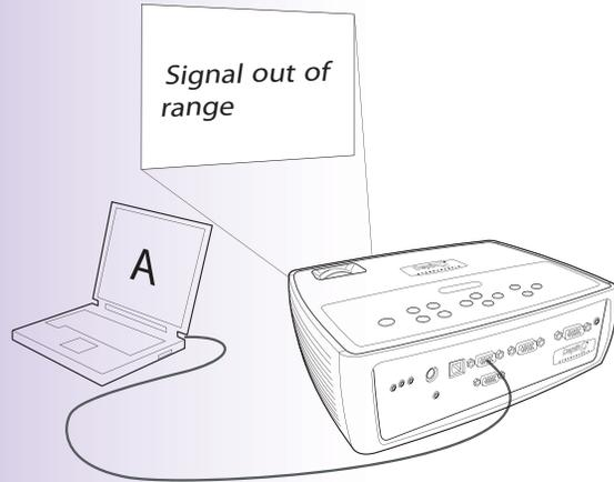
press the Auto Image button on keypad to re-sync
