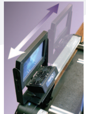
Optional two position actuator allows automatable switching between 2D and 3D.
